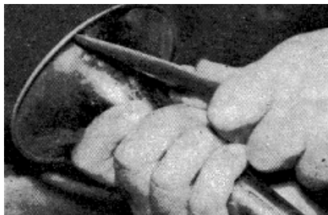
Using tip of burnisher to remove rim dents.
